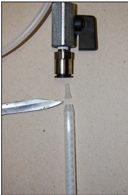
Cut static mixer as shown before inserting into valve assembly.
